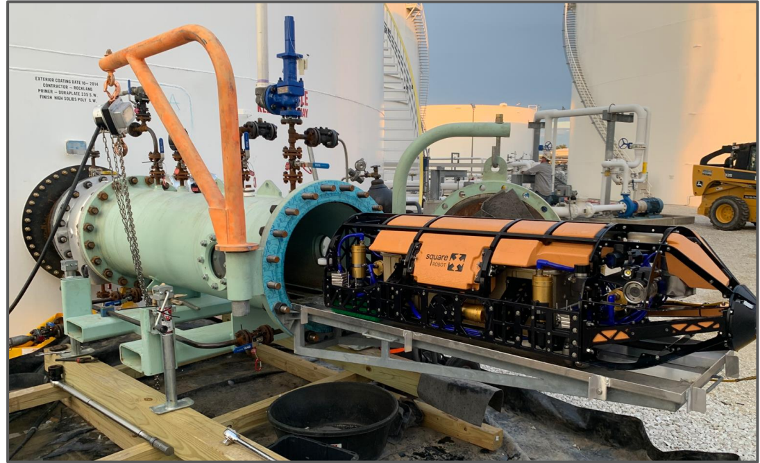
Vehicle Chamber 24" Gate Valve Manway Adapter
