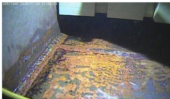
Figure 22 - PAUT Scanning Bottom against Tank Shell during APS in Isononyl Alcohol
