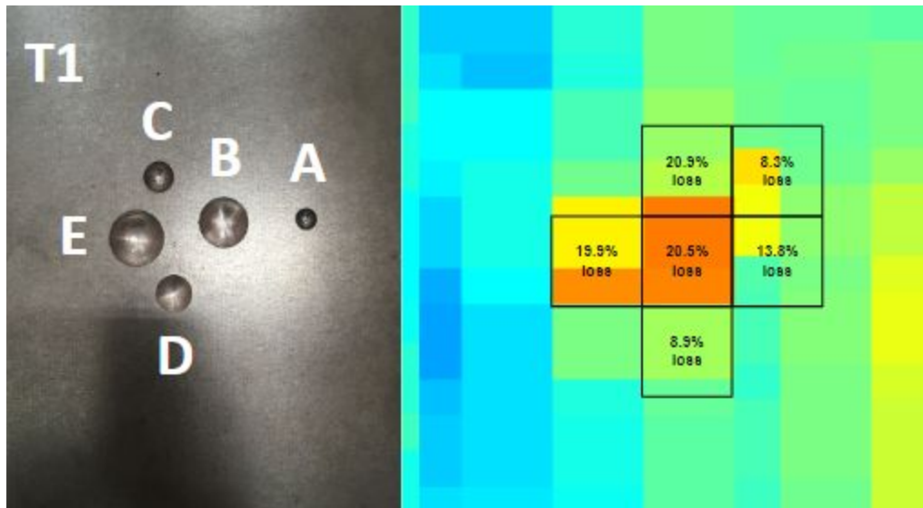
Figure 27 - PEC Results, Product Side Scan, Defect Group T1
