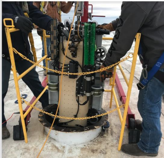
Robot Recovery through Manway; Decontamination Process
