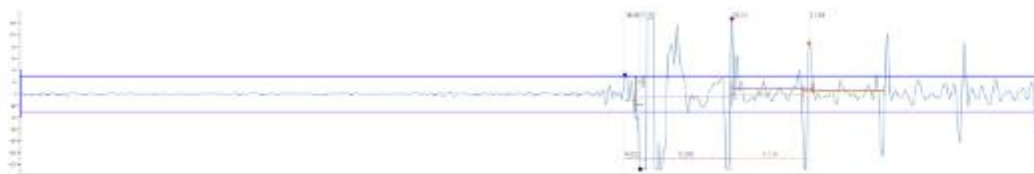
Figure 8 - A-Scan reading 0.249-inch
