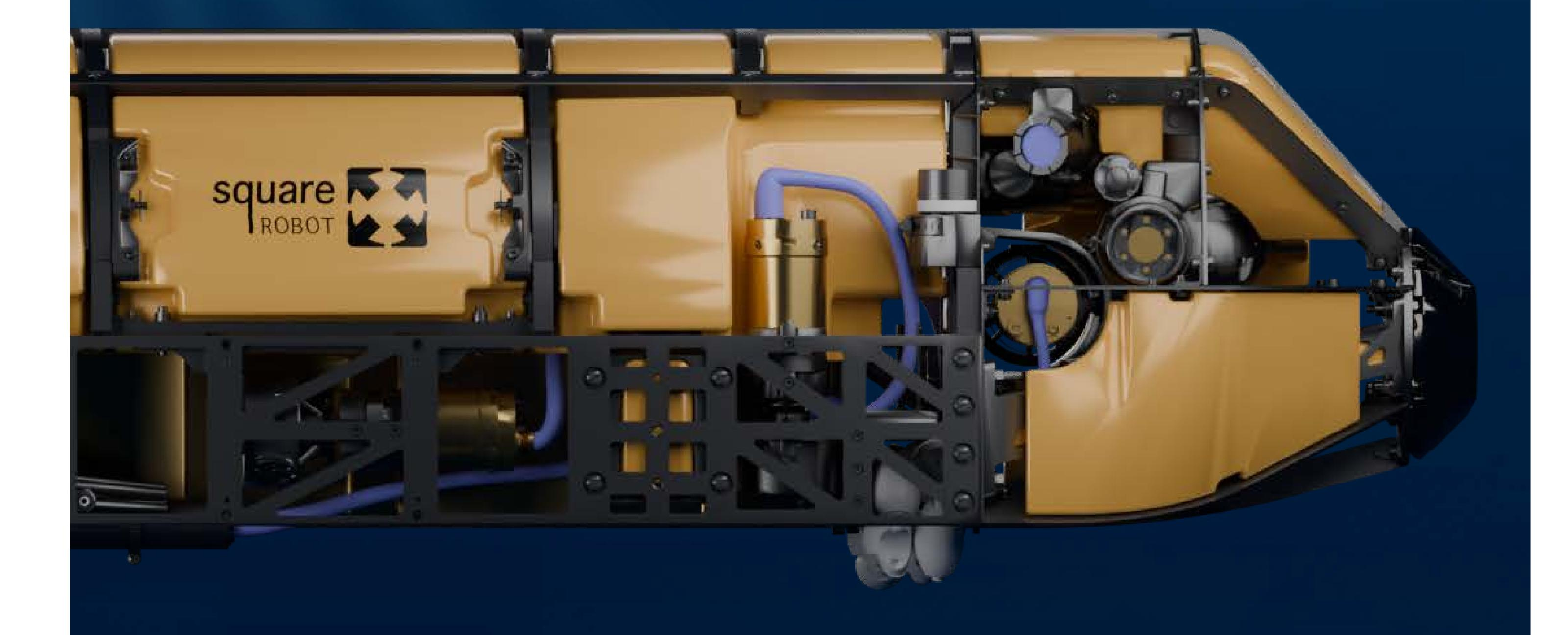
Square Robot's autonomous, submersible robots and advanced inspection technology enable safe, informed above-ground storage tank utilization by eliminating the need to take tanks containing volatile products including diesel, jet fuel, and gasoline out of service for required internal inspection,
