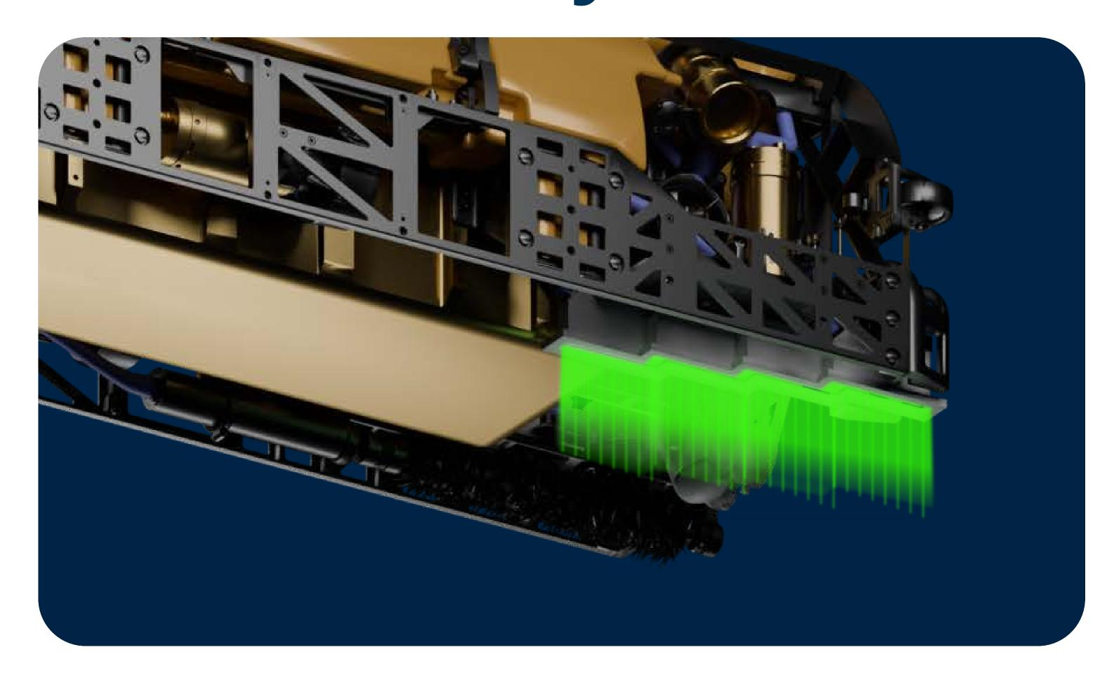
The robotic systems are engineered for optimal inspection of tank bottoms, focusing on the critical zone near the tank shell where corrosion can cause major failures.
