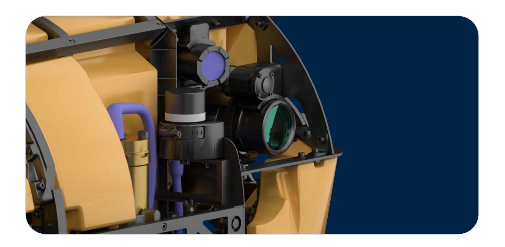
Multi-directional views from the high-resolution cameras allow the robot to record visual datasets on the condition of internal coating, structures, nozzles, and sediment accumulation levels. Our robot correlates its position in the tank with Phased Array Ultrasonic Testing and high-resolution visual data of the same location.
